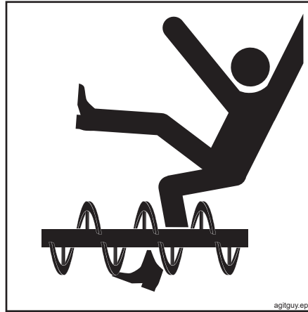
Figure 84 Lifting hopper grate exposes the agitator and the concrete valve
