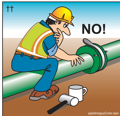
Figure 81 Never straddle or sit on a pressurized pipeline
