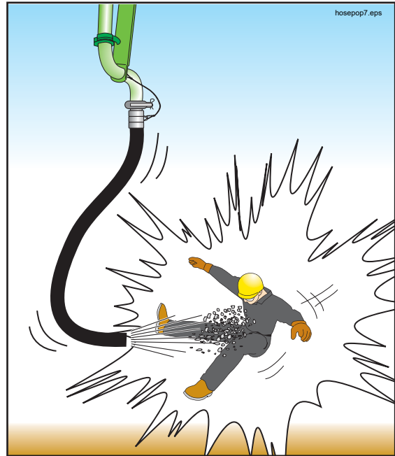
Figure 90 Stay away from the point of discharge when starting or restarting, and when there's air in the pipeline
